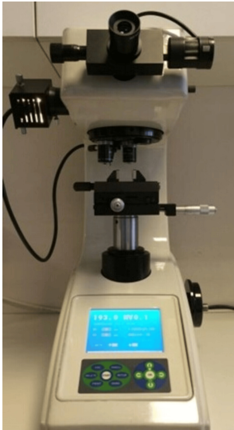
FIGURE 1: Application of Vickers diamond tip to samples in microhardness tester
