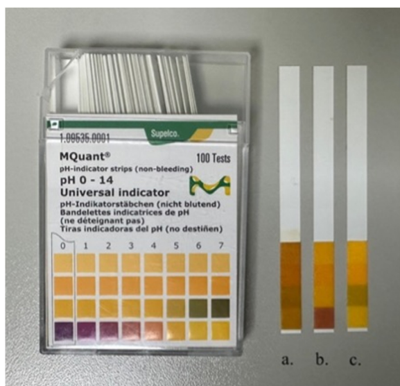
Fig 4. The pH of the solutions was measured with MQuant pH indicator strips. a , Coffee; b , Cola; c , Distilled water.
