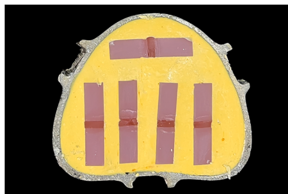
Fig. 2A. The specimen with a 3 mm wax section was placed in the dental flasks.
