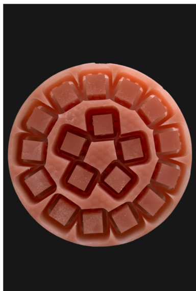
Fig. 1. IvoBase CAD PMMA disk after subtractive manufacturing, showing the milled denture base specimens.
