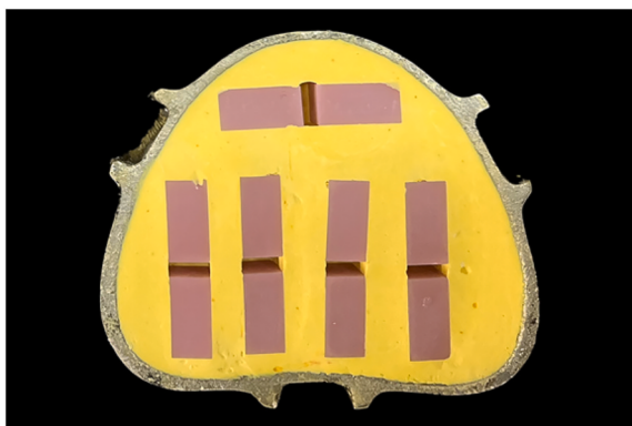
Fig. 2B. 3 mm section removed and ready for soft lining reconnection.
