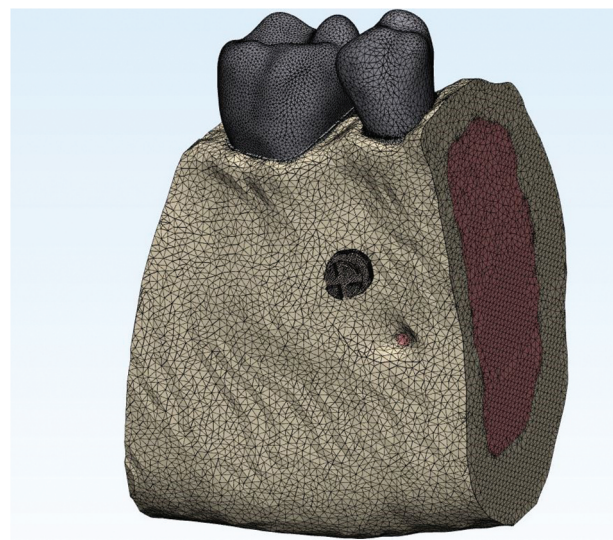
Figure 1. Finite element model consisting of separately modelled; miniscrew, tooth, PDL and cortical and cancellous bone elements.
