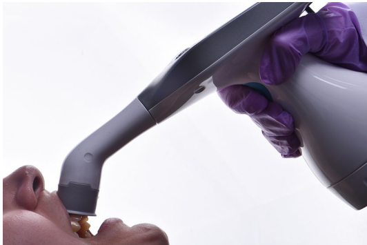
Fig. 1 Clinical dental color measurements with RayPlicker (Borea, France)
