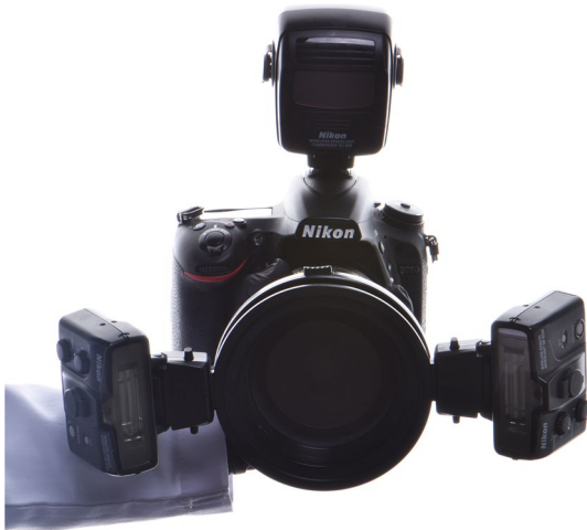
Fig. 2 Digital dental photography kit (D750 body, R1C1 Speedlight SB-R200 flash, 105 mm AF-S Micro Nikkor VR lens, Nikon, Japan)
