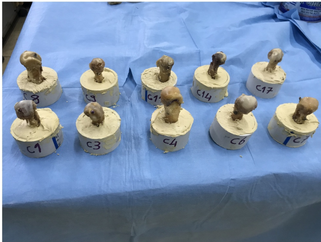
FIGURE 3 Metatarsals with their proximal ends embedded in PVC pipes with steel putty and their distal ends left exposed.
